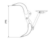
\*To aid in mounting, center pins are sleeved to hold grapple together.
